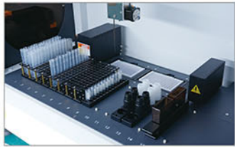
Sample & Reagent & Dilution Rack Module Original sample tubes available; Rack positions programmable.
